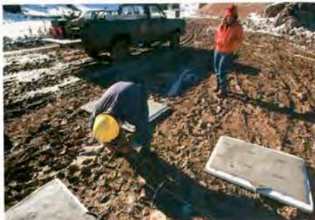
A technician hooks up detonating cord attached to "sandwiches" of molds, metal and explosives in desert.
