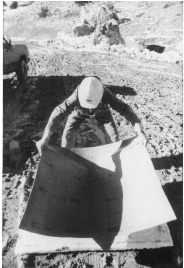
Fig. 4. Preparations for a blast: the C1 Datasheet glued to a rubber mat is placed on the plaster mold by a technician. Twenty pounds of plastic explosives will make four plates measuring 3 × 4 ft.
